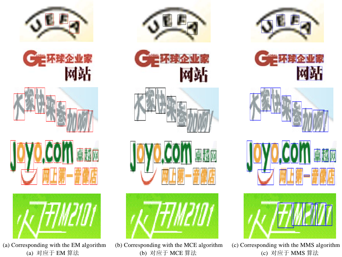
Fig.1 The illustration of different text extraction results corresponding with three training methods (extracted texts are contained in the rectangles)
