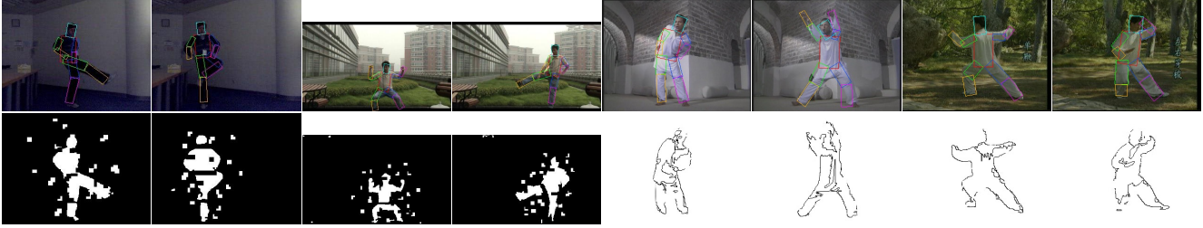
Figure 14. Some estimation results on noisy foreground or edge map (first row: results, second row: associated foregrounds or edge maps)
