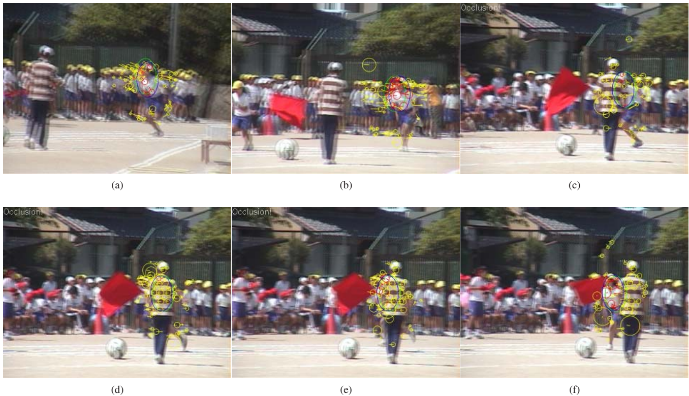
Figure 5: Challenging situations including appearance changes, background clutter and occlusion. Tracking results of frames 77, 81, 89, 91, 92 and 93 are shown. In each sub-figure, background features are denoted by yellow circles, and object features are red circles. Green and blue ellipses stand for object position in previous frame and current frame, respectively. Here, An area ratio based occlusion indicator is used to response with occlusion, as shown in frames 89, 91, 92.
