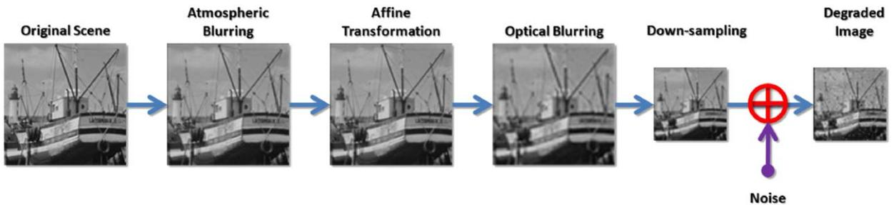
Fig. 1. The block diagram of an imaging system.
