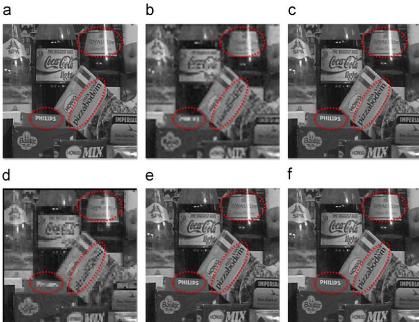
**Fig. 7.** Comparison of reconstruction results of image Shopping, when pixels are insufficient: (a) original image, (b) LR image, (c) bi-cubic, (d)  $L_1$ +BTV, (e)  $L_1$ +ABTV, and (f)  $L_1$ +ABTV+CG.
