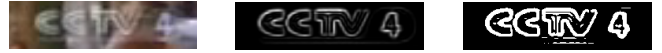
Fig. 2. TV logo detection (Left to right: the original logo image, the gray-level image, and the logo’s binary mask by OSTU)
