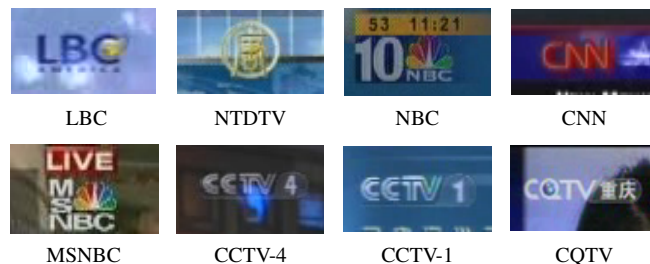
Fig. 1. Examples of the magnified TV logo images(LBC, NTDTV, NBC, CNN and MSNBC are opaque logos; CCTV-4 and CCTV-1 are semi-transparent logos; CQTV is an animated logo.)
